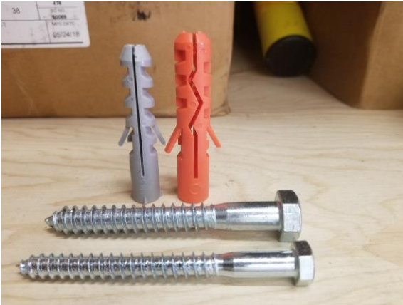
Figure 13. The orange sleeves and longer (4") bolts work better than the grey sleeves and shorter bolts that are included with the bumps.
