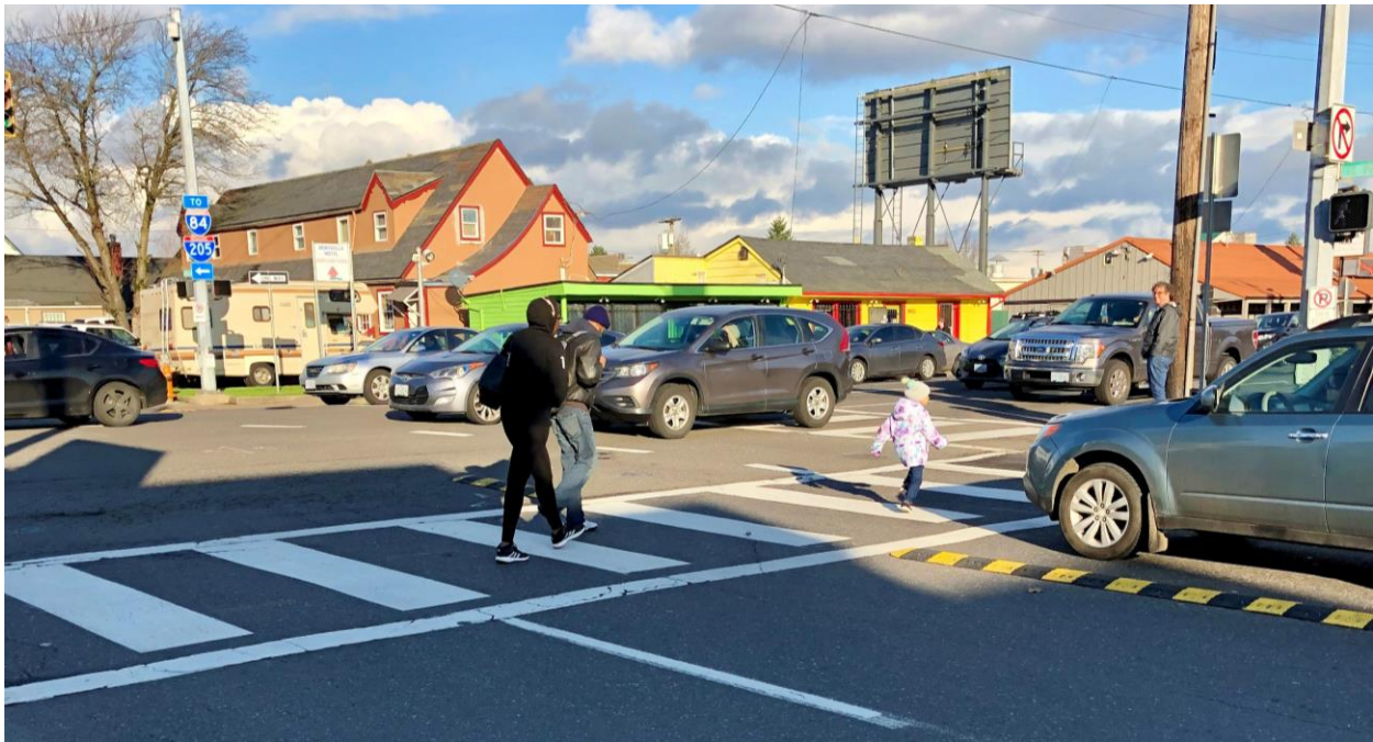
Figure 4. A hardened centerline using bumps with a nose at SE 99 th Avenue & Stark Street, looking northeast, on December 23, 2019.
